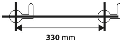
3. Use a drill to drill the mounting holes. Use a 6 mm drill bit for drilling. The depth of the holes must be at least 26 mm deep. Do not use a smaller size!
